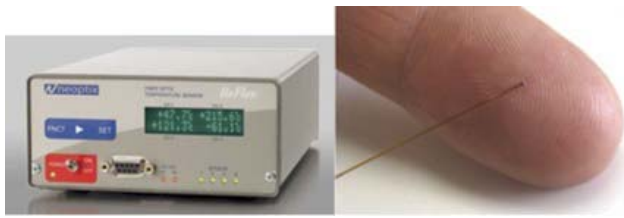
Figure 1. Fiber-optic system. The system consists of the measuring unit (left panel) and the fiber-optic temperature sensor (right panel). The bare fiber-optic temperature sensor is 300 microns in diameter (right panel).
