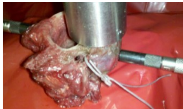
Fig. 3. Experimental Set-up for Intact Cervical Spine. The anterior sensor measures anterior bulge, the posterior sensor tracks the displacement of the bone movement.
