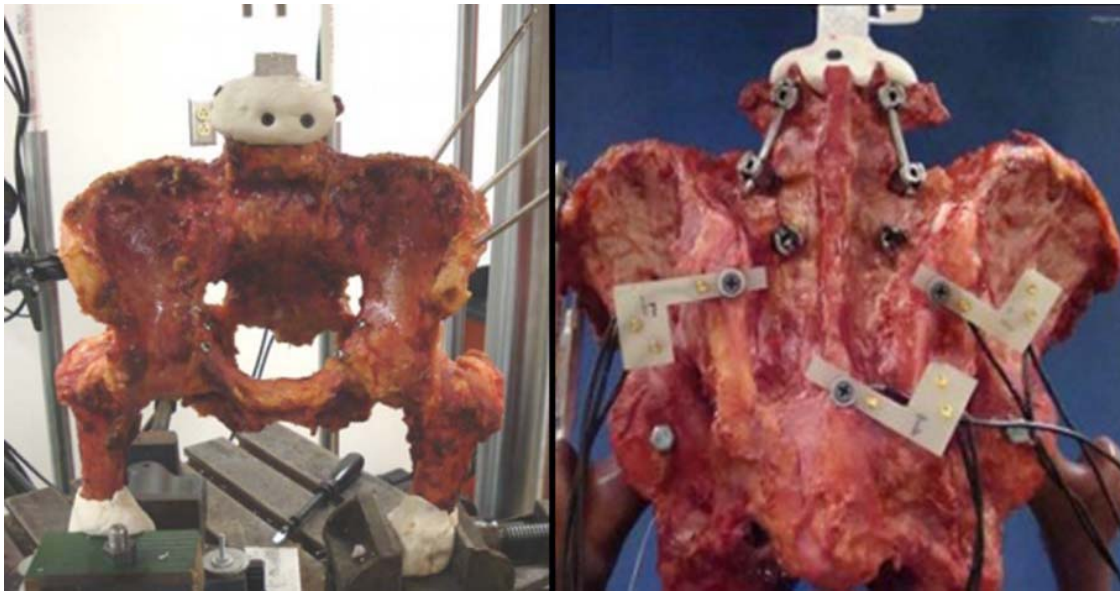
Figure 7. Biomechanical study on intact sacroiliac joint, double-leg stance model (left) and posterior view after L4-L5 fusion (right). 44
