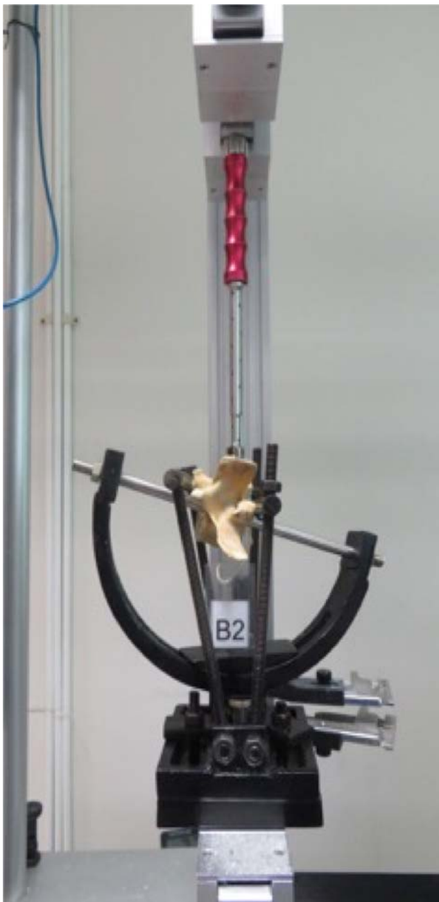
Figure 5. Pull-out testing. The screw is connected to the insertion screwdriver in the apparatus that was designed to hold the vertebrae and the screw in line with the machine. The screw was then pulled out in the direction of the insertion.
