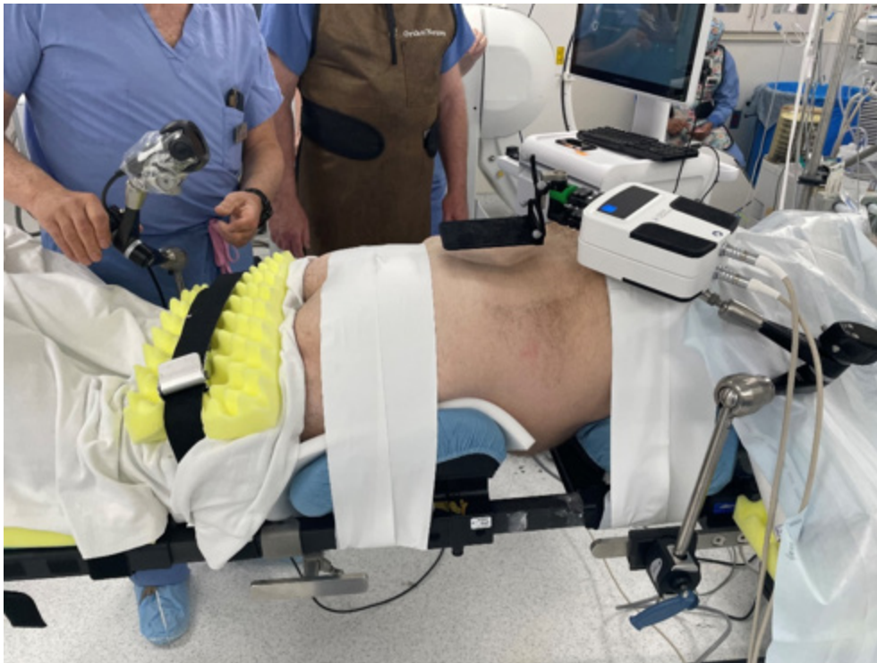
Figure 1. Operating room (OR) setup. The robot is mounted on the surgeon's side of the table just below the patient's axilla, and the camera is mounted on the opposite side of the OR table at the patient's midthigh level and positioned so that the camera view is directed cranially and along the patient's midline.
