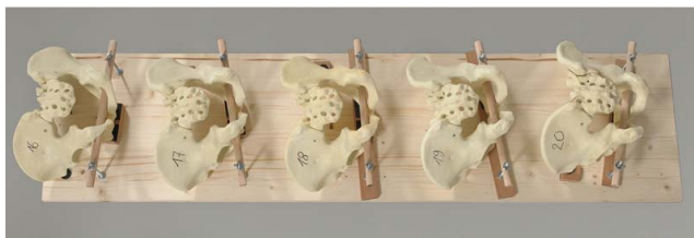
Figure 1. Pelvic models mounted to a wooden board with different angulations and tilts.
