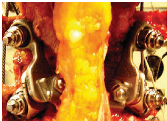
In vitro testing of Anatomic Facet Replacement System-repaired spine segment. The supraspinous ligament and majority of the interspinous ligament were left intact.
