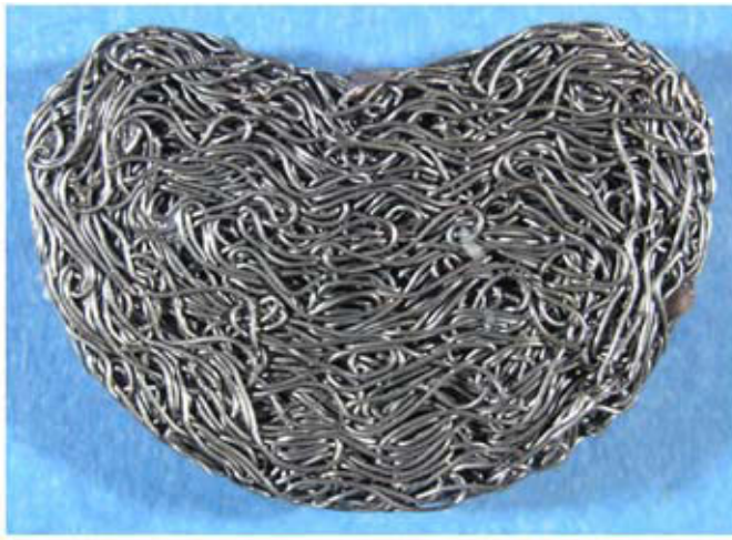
New nucleus prosthesis made of knitted titanium filaments.
