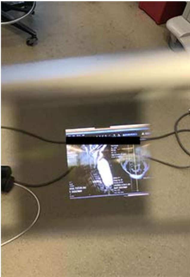
Figure 2. View of the image that is displayed within the augmented reality heads-up display (AR-HUD) system as seen from the operator's perspective (black line is not on actual display; it is only used to cover up patient identity).
