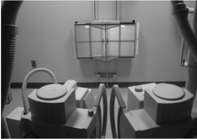
RSA examination was performed in a specialized radiographic suite with double roentgen tubes directed in 40° diverging lines.
