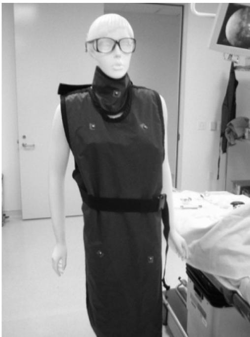
Fig. 1. Mannequin with dosimeters.
